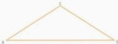
$$\overline{bc}^2 = \overline{ab}^2 + \overline{ac}^2 - 2 \cdot \overline{ab} \cdot \overline{ac} \cdot \cos \hat{a}$$
