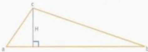
$$\text{sen } \hat{a} = \frac{H}{\overline{ac}} \quad \wedge \quad \text{sen } \hat{b} = \frac{H}{\overline{bc}}$$
